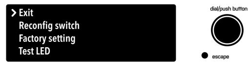
Rotate the data button to move the cursor to the desired option. Press the data button to confirm your choice. The VLAN-toolbox will then perform the selected action.
