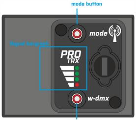
For the DMX operation, turn off the W-DMX module by holding the MODE button. Both W-DMX and MODE buttons light in red color.
