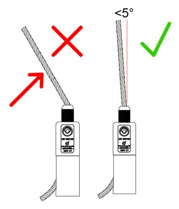
The wire rope must exit in line with the Cable Holder.
