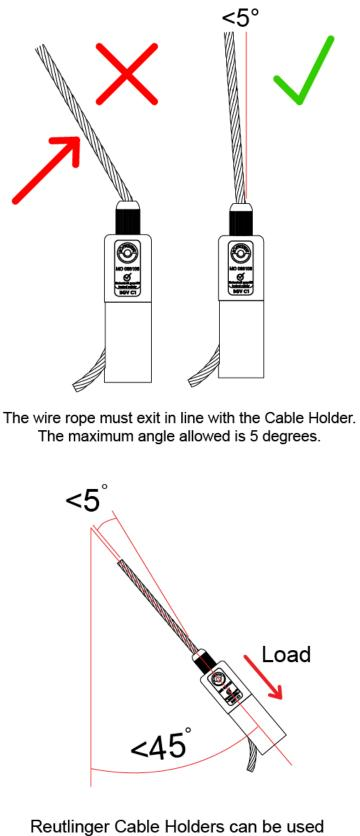
Reutlinger Cable Holders can be used up to an angle of 45 degrees.
