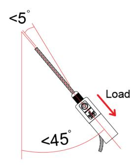
Reutlinger Cable Holders can be used up to an angle of 45 degrees.
