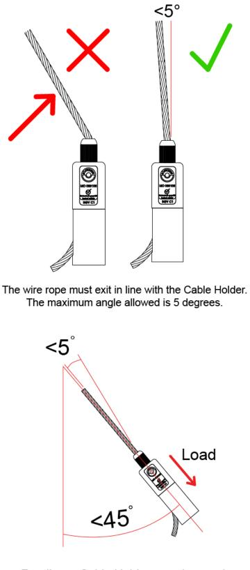
Reutlinger Cable Holders can be used up to an angle of 45 degrees.
